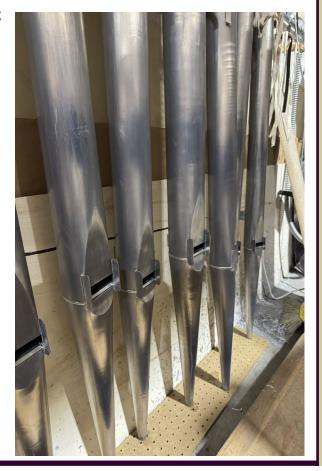
Right: The English Diapason basses pipes that have been made, racked, washed, and buffed. These pipes will be installed in the façade in the Chancel opening.
